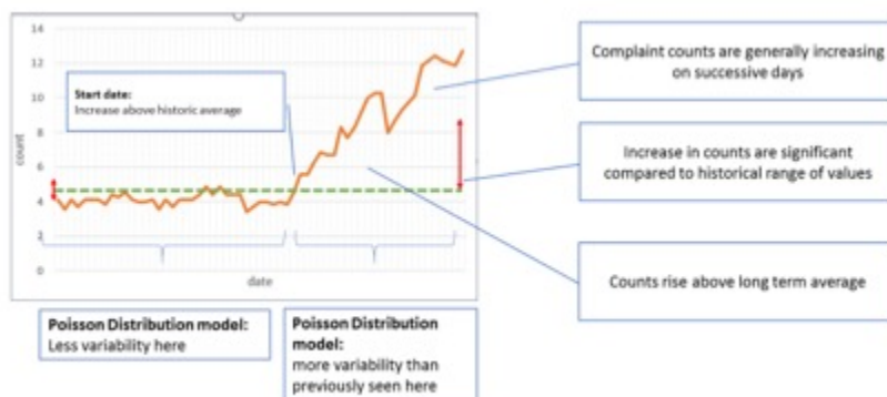
Figure 31: Diagram showing the trend detection rule
